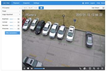
Adjust camera direction and lens angle (Direction: horizontal 205°, vertical 70°) till the live image in IPCWeb reaches requirements.
