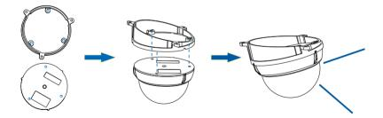
3. Refer to the steps of Ceiling Mount to finish the installation of slant base bracket.
